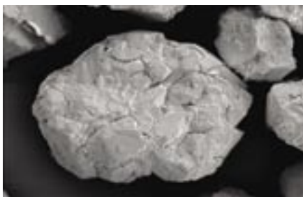
Sand particles unaffected by hardened deposits
